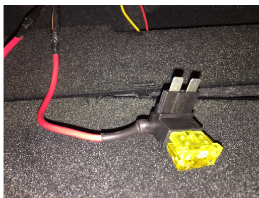
Add-a-fuse piggyback fuse holder from eBay.
